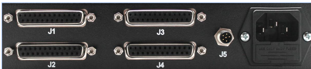
Figure 1-6: RICI 5000 Model 010-10 Rear Panel (100-240VAC), Revision D or Earlier
