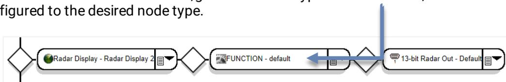
Inserting a node is valid only on the diamond connectors after an input type node. The **Insert a function** selection is unavailable and greyed out before an input node and on the last diamond connector of a merged data path.
