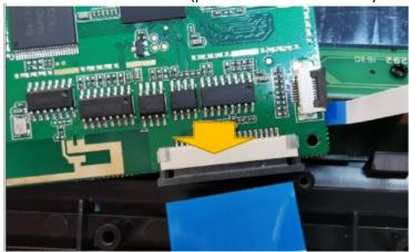
3. Disconnect the second ribbon cable from the PCB board by flipping the black notch indicated by the yellow arrow away from the PCB.
